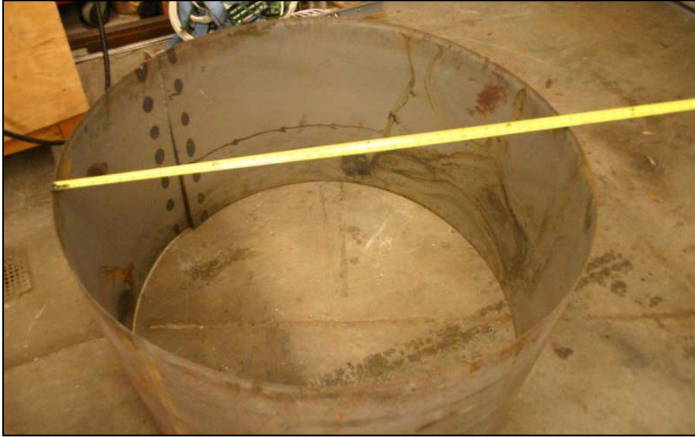
Figure A.1. Steel testing form, 42-inches in diameter.
