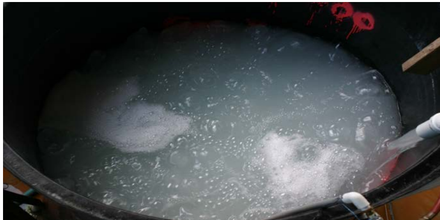
Figure 3.10. 60 sec/qt polymer slurry after mixing being agitated with bubbler system.
