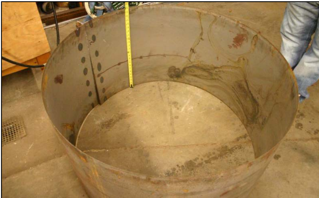
Figure A.2. Steel testing form, 24-inches in height.
