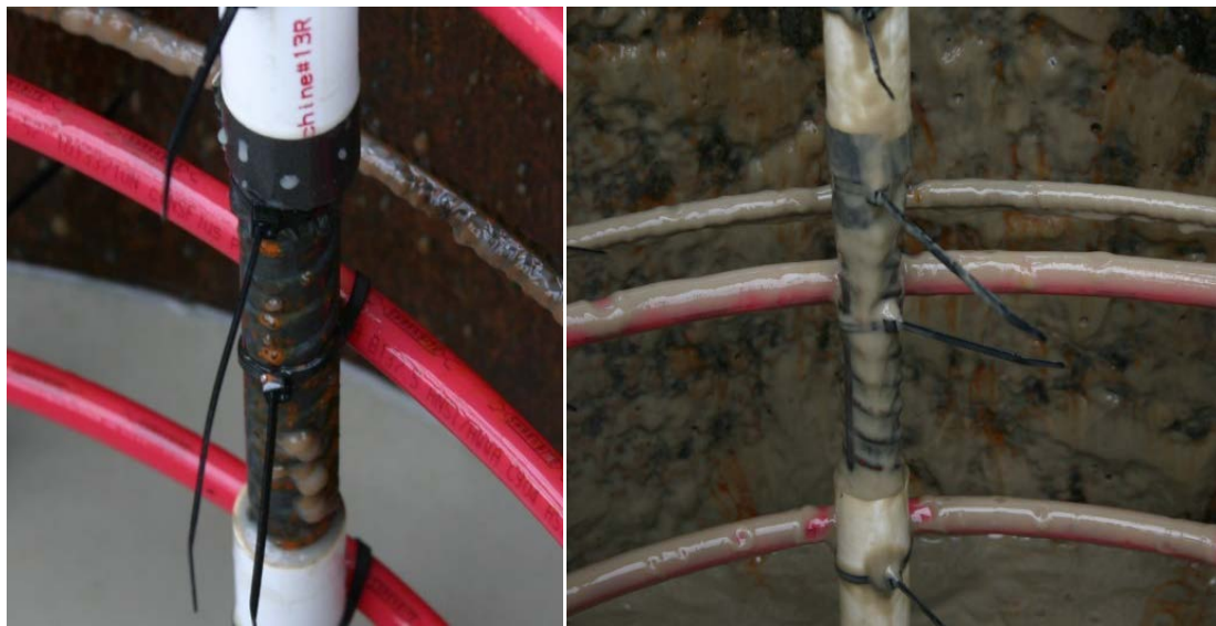
Figure 5.3. Residual slurry noticed on reinforcement 30 second (left), 90 second (right).
