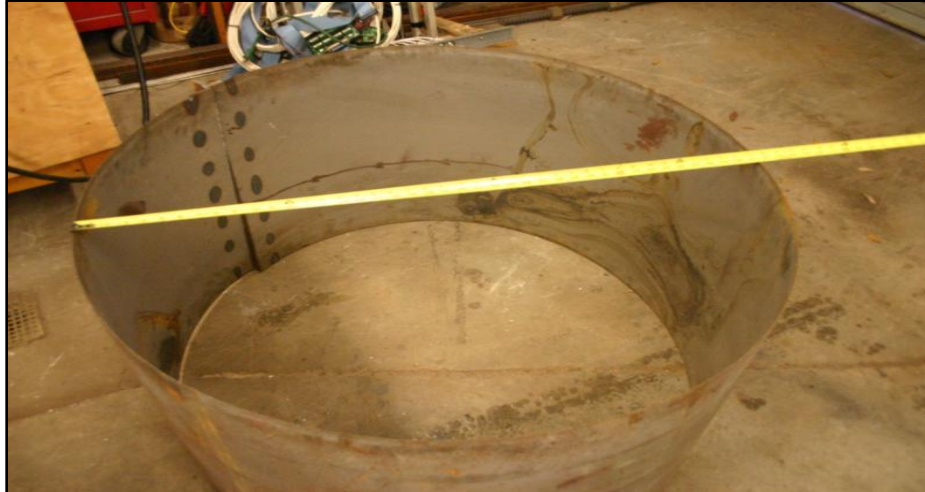
Figure 3.3. 18 gauge steel rolled to 42-inch diameter.
