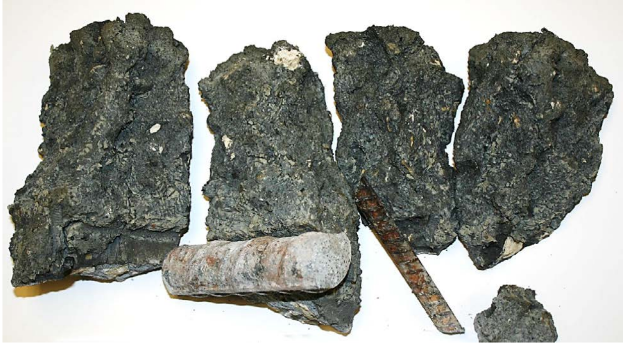
Figure 5.11. Encapsulated slurry in 50 sec/qt shaft core.
