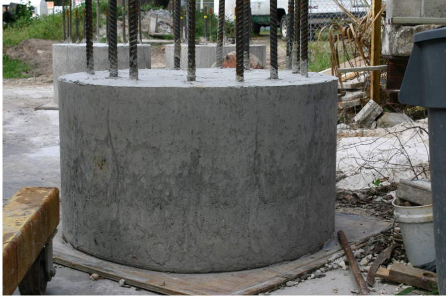
Figure A.26. Shaft 17, 85 sec/qt polymer slurry after pressure washing.
