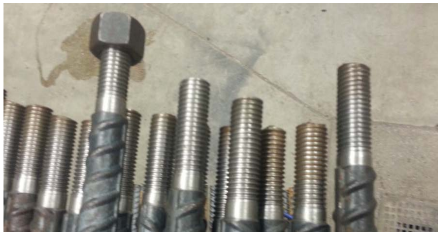
Figure 3.7. Reinforcement after machining.
