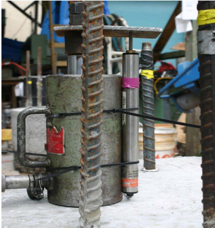
Figure 3.15. Ram configuration during pullout testing with LVDT in place.
