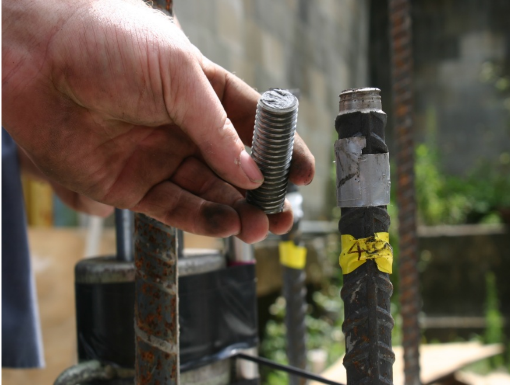
Figure A.34. Bar failure from shaft 6, water.
